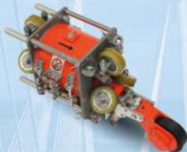
INTROS Magnetic Head MH 60-85. For bridge cables, offshore cranes.
