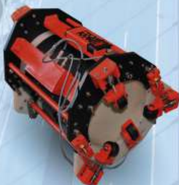
INTROS Electromagnetic Head EH-300. For bridge cables with parallel strands.
