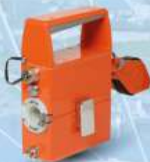
INTROS Magnetic Head MH 6-24. For elevators, cableways, cranes.
